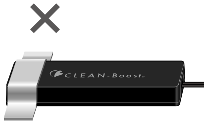
Figure 1 Do Not Shield Antenna Section
